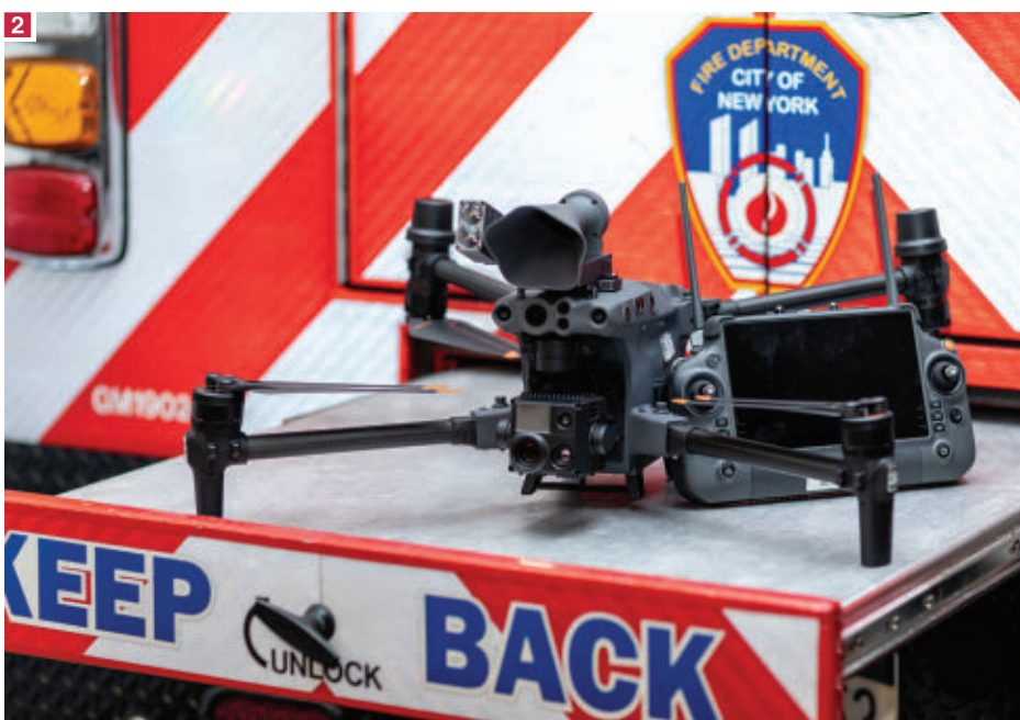
1 The FDNY uses its drones on structure fires to locate hot spots as well as identify which way a fire is moving. (Photos 1-2 courtesy of the Fire Department of New York.)
