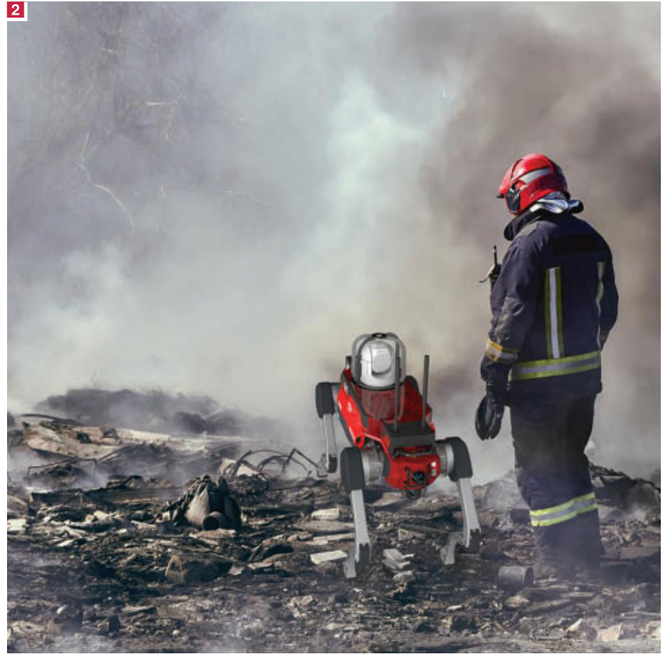
2 Robot dogs equipped with gas sensors can measure the concentration of toxic gases in the air in real time, transmitting data to command posts for early fire assessment and containment of toxic gas leaks.
