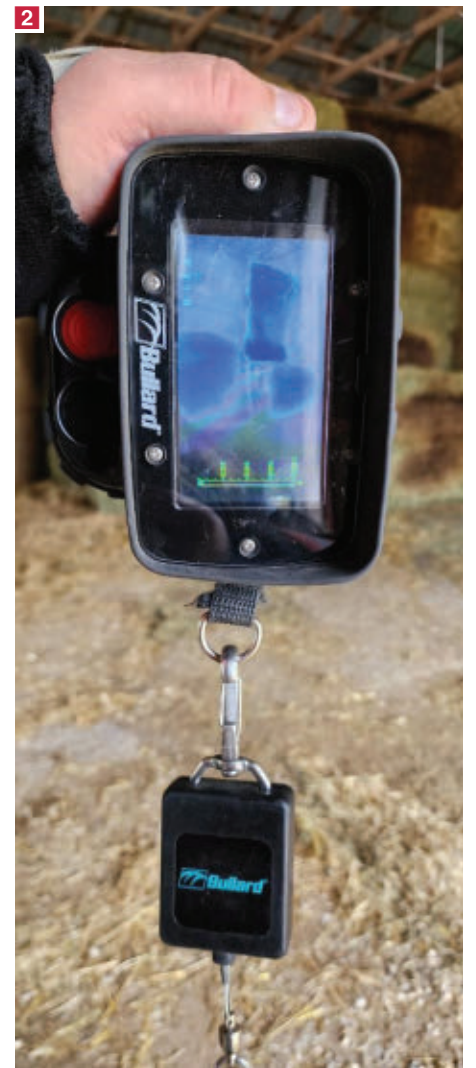
2 TI assessment after extinguishing burning hay bales. [Photo courtesy of West Grey (Ontario, Canada) Fire Services.]
