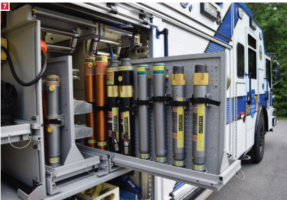
5 The squad's battery-powered blowers and saws. 6 The Walkersville rescue's cribbing compartment. 7 These slide-outs carry the rig's Paratech rescue struts.
