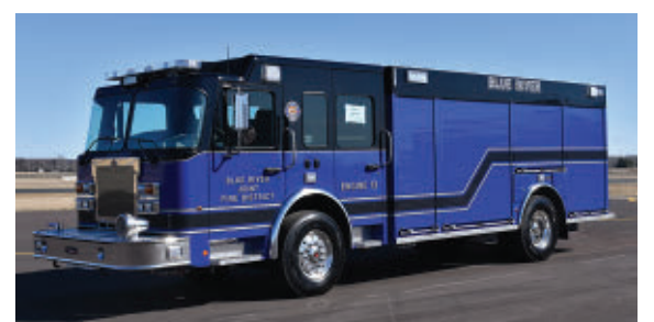
CUSTOMFIRE —Blue River (WI) Fire & Rescue pumper. Spartan FC-94 cab and chassis; Cummins L9 450-hp engine; Waterous S-100D 1,500-gpm pump; UPF Poly 1,780-gallon polypropylene water tank; 20-gallon foam cell; FoamPro 1600 Class A foam system; pull-out tool boards with locking mechanism; front bumper storage well. Dealer: Wayde Kirvida, CustomFIRE Apparatus, Osceola, WI.
