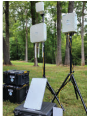
The RUCS unit + distribution modules send signals 1000'.
