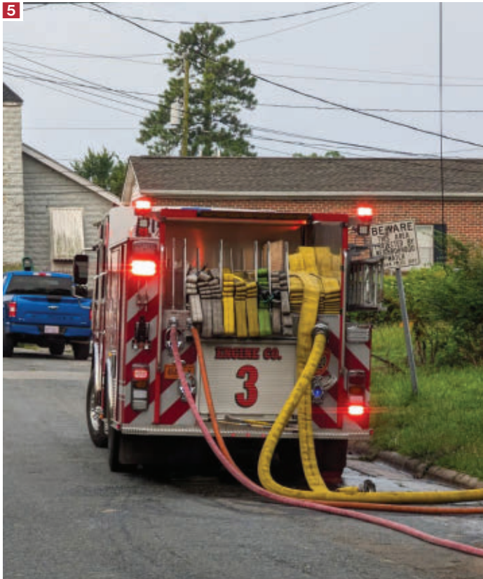
4 One of the requirements that Durham Fire had in its pumper specs was low hosebeds. 5 Most of the hoselines on Durham's Sutphen pumpers come off the rear of the vehicle, as shown here at a working fire scene.
