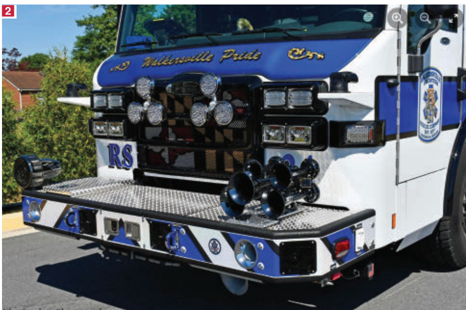
1 The Walkersville (MD) Volunteer Rescue Company's Pierce Velocity walk-around heavy rescue. (Photos 1-2 by Mike Sanders.) 2 The rescue truck has twin Roto-Rays, a Federal Q, two electronic siren speakers, twin air horns, and a set of train horns. 3 The new rig's booster line, pump panel, and controls for lighting masts. (Photos 3-8 courtesy of First Due Apparatus Solutions.) 4 The rescue truck carries AMKUS extrication tools mounted on lazy Susan mounts and DeWalt battery chargers.
