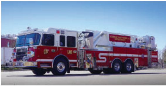
LADDER TOWER —Surprise (AZ) Fire Medical Department platform aerial. Spartan Gladiator MFD cab and chassis with 10-inch raised roof with Advanced Occupant Protection System cab and chassis; Cummins X15 605-hp engine; Ladder Tower five-section steel aerial ladder with 1,000-pound platform rating; TFT Monsoon monitor; formed aluminum body; Harrison 8-kW generator; Duo-Safety ground ladders. Dealer: Tim Burkhart, Spartan ER, Brandon, SD.
