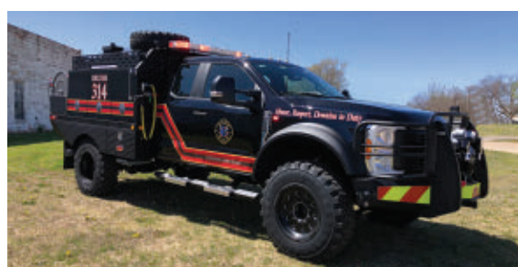
WEIS FIRE AND SAFETY EQUIPMENT —Lexington County (SC) Fire & Rescue two Quick Attack units. Ford F-550 Super Cabs and chassis; 6.7L 500-hp diesel engines; Darley 2BE-with 24K Kubota engines; 300-gpm @ 75-psi pumps; UPF Poly 400-gallon water tanks; 12-gallon foam cells; rear pump controls; TFT Tornado front monitors; Trident Foamate model 31 Class A foam systems; front ground sweeps. Dealer: Weis Fire and Safety Equipment, Salina, KS.
