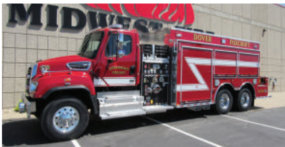
MIDWEST FIRE —Dover-Foxcroft (ME) Fire Department pumper-tanker. Freightliner 114SD cab and chassis; Cummins X12 500-hp engine; Waterous CSU 1,250-gpm pump; APR polypropylene 3,000-gallon water tank; three Newton 10-inch stainless steel dump valves with telescoping chutes; All-Poly™ construction; "Sweep Out" style compartments. Dealer: Newt Johnson, Midwest Fire, Luverne, MN.
