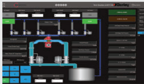
Mounted on movable carts, the new control screen allows test technicians to adjust the RPM, ball valve, and suction valves while working on other duties.
