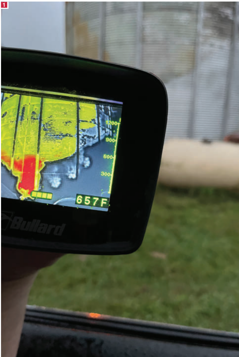
1 Monitoring excessive heat from a silo fire with a TI. [Photo courtesy of Harrison County (KY) Fire Department.]
