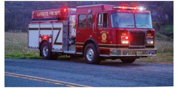
FOUTS FIRE —Lafayette Fire Department, Lafayette Township, NJ, FB-94 rescue-pumper. Spartan FC-94 cab and chassis; Cummins L9 380-hp engine; Hale Qmax 1,500-gpm pump; UPF Poly 1,000-gallon water tank; Alco-Lite ground ladders. Dealer: Fred Reader, Firefighter One Apparatus, Sparta, NJ.
