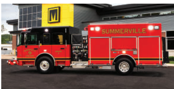
MARION —Summerville (GA) Fire Department pumper. Spartan Metro Star cab and chassis; Cummins X12 500-hp engine; Waterous CSU 1,500-gpm pump; UPF Poly 1,000-gallon water tank. Dealer: Chuck Miller, Fearless Flames Inc., Canton, GA.
