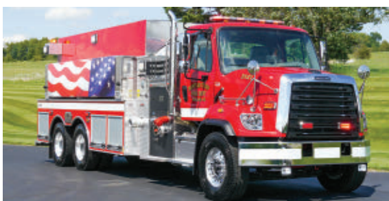
FIROVAC —Mifflin Township Fire Department, Ashland, OH, pumper-tanker. Freightliner 108SD cab and chassis; Cummins L9 400-hp engine; Darley PSP 1,500-gpm pump; 3,000-gallon aluminum water tank; Eagle body; Firovac power swing down portable tank bracket holding two 3,000-gallon Husky portable water tanks. Dealer: Larry Reber and Brian Stoffer, Fireovac Power Systems, Apple Creek, OH.
