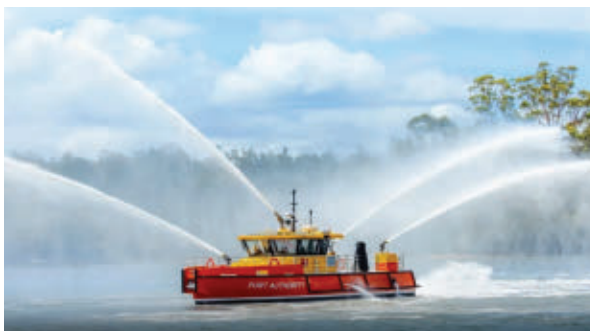
Two new firefighting vessels for New South Wales are equipped with two Darley PSP 2000 pumps, flowing over 5000 GPM.
