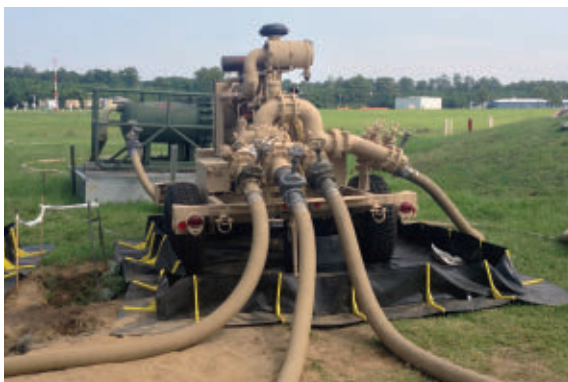
At the heart of the E2FDS is a modified version of our LE600 pump.
