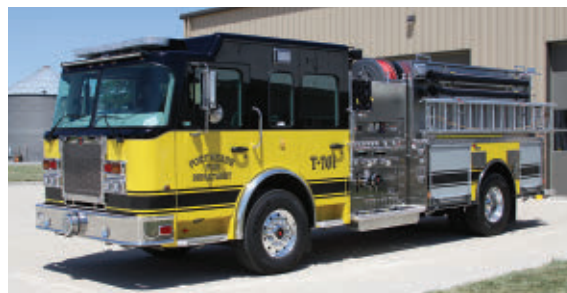
TOYNE —Fort Meade (FL) Fire Department pumper-tanker. Spartan FC-94 cab and chassis with 10-inch raised roof; Cummins L9 450-hp engine; stainless steel body; Hale Qmax-XS 1,250-gpm pump; UPF Poly 1,800-gallon water tank; 30-gallon foam cell; FoamPro 1600 Class A foam system; Akron Apollo Hi-Riser monitor; Syntex 2,100-gallon portable tank; Zico hydraulic Porta-Tank rack; Duo-Safety ground ladders. Dealer: Royce Holton, Tactical Fire, Winder, GA.
