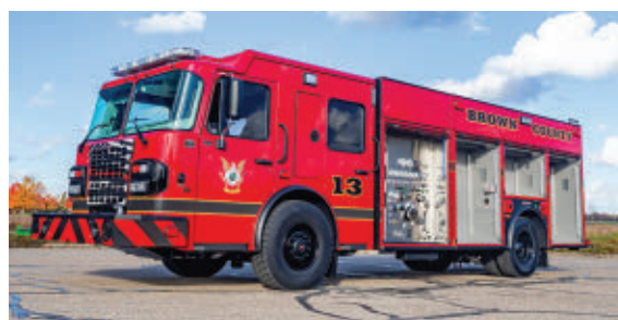
SPENCER MANUFACTURING —Brown County Volunteer Fire Department, Nashville, IN, pumper. Spartan Metro Star MFD cab and chassis; Cummins L9 450-hp engine; Hale Qmax 1,500-gpm pump; UPF Poly 1,000-gallon water tank; Smart Power 8-kW generator; Alco-Lite ground ladders. Dealer: Shane Scott, The Fire Department Connection, Shelbyville, IN.
