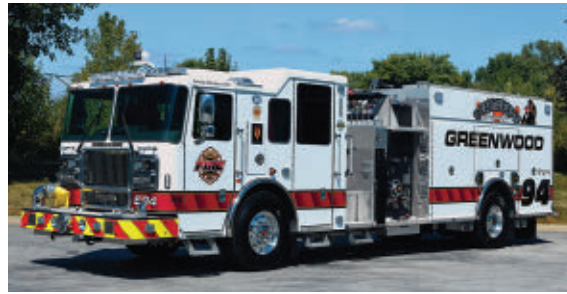
SEAGRAVE —Greenwood (IN) Fire Department pumper. Marauder stainless steel tilt cab and chassis; Cummins X12 500-hp engine; Waterous CMU 1,250-gpm pump; 750-gallon polypropylene water tank; Harrison Stinger 6-kW generator; Duo-Safety ground ladders. Dealer: Kyle Koons, 911 Fleet and Fire Equipment, Worthington, IN. (Photo by Kent Parish.)
