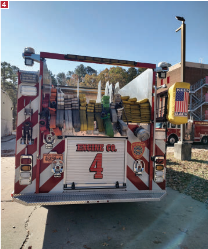
4 One of the requirements that Durham Fire had in its pumper specs was low hosebeds. 5 Most of the hoselines on Durham's Sutphen pumpers come off the rear of the vehicle, as shown here at a working fire scene.
