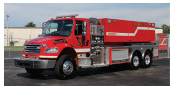
FIRE MASTER —Beggs (OK) Fire Department pumper-tanker. Freightliner M2 106 cab and chassis; Cummins L9 350-hp engine; Hale Qflo 1,250-gpm pump; Pro Poly 3,000-gallon polypropylene water tank. Dealer: Steve Loftin, Fire Master, Tulsa, OK.
