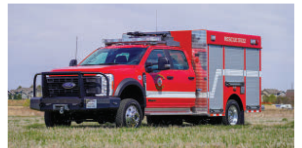
SVI TRUCKS —Sugar Loaf Fire Protection District, Boulder, CO, light rescue. Ford F-550 four-door cab and 4x4 chassis; 6.7L Power Stroke V8 Turbo 475-hp diesel engine; 9-foot walk-around rescue body; Command Light Knight KL415D-W2, 4 Whelen Pioneer Plus PFH2S light tower; OnScene Solutions transverse heavy-duty cargo slides; Ramsey RE-1200R heavy-duty winch. Dealer: Jason Kline, SVI Trucks, Fort Collins, CO.
