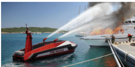
The Zycraft remote controlled unmanned fire fighting vessel.
